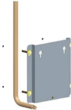
02. Fix 2 x M6\*10 screws to the back of the EV Charger and hang on the backplate.
