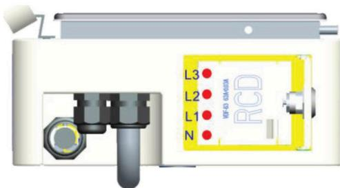
02. Connect the power wires to the terminal board, and make sure that the PE cable passes through the CT clamp.
