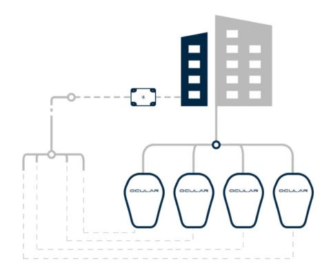
Load Management protects the building's electrical infrastructure, eliminates the risk of overloading, ensures efficient operation for all EV chargers within limited power sources, and saves costs for upgrading the electrical infrastructure and electricity bills. The Ocular range have advanced load management features, making them the ideal solution for all electric vehicles across Australia
